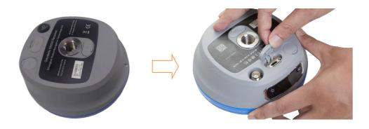
Insert the SIM card with the contacts facing upward, as indicated by the SIM card icon next to the SIM card slot.
